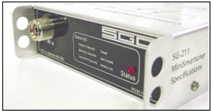
Photo F— The SG-211 MiniSmartuner is designed to meet professional and amateur needs for a lightweight, portable antenna coupler for low-power applications, one which requires no external battery support. The SG-211 handles from 1 to 60 watts of input power over a frequency range of 1.8 to 60 MHz. (Photo courtesy of SGC)
