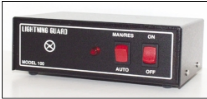
Photo E— The Lightning Guard Model 100 from Electronic Specialty Products is designed to protect your transceiver from lightning when you are out of the shack. AC power, as well as your antenna coax, connect to the Lightning Guard so that your transceiver gets its AC power and its antenna connection through the Lightning Guard. (Photo courtesy of Electronic Specialty Products)
