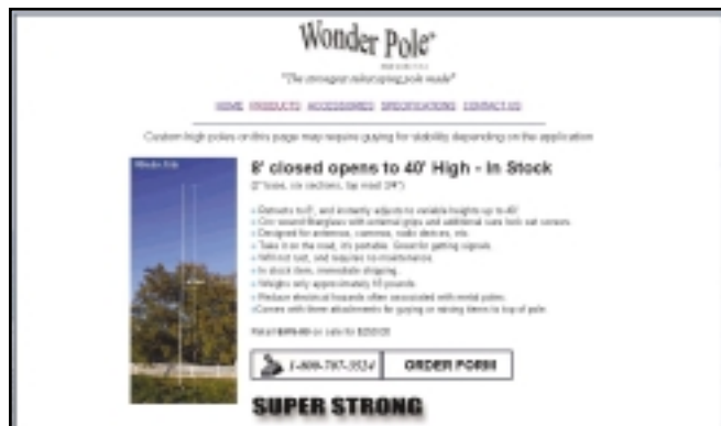
Fig. 2—The American Flag & Banner Co. makes a number of highly portable, super-strong telescoping poles under the Wonder Pole® name, several of which have excellent potential for amateur use. Available in several different sizes and configurations, the telescoping poles are made from sections of six-ply fiberglass tubing. (Graphic from the Wonder Pole website)
